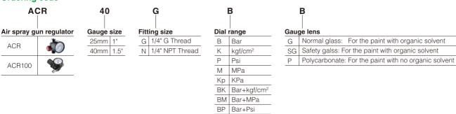
Note: ACR air regulator is a control valve which through adjusting the discharge area to regulate the flow rate. ACR100 It's a pressure regulator. Not for limiting the air flow rate .
